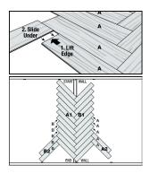
7. Starting with the last full plank at the end wall, continue installing sequential columns (Column "A2" and "B2"). Lift the untapped edge and slide the new plank under, as pictured on the right. Position the tongue and groove of the first plank in column "A2" into place with the last plank in column "B1". Tap seams to completely lock planks.
