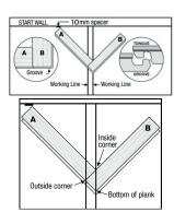
5. You have now created your "starting V". Slide the "starting V" against the wall. The working lines should meet up with the plank as shown on the right. Plank "A" should be placed closest to the wall, touching the 10mm spacer. Plank "B" will be offset, this is normal. The proper alignment of the "starting V" is critical for installation.
