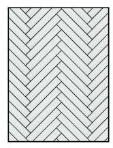
This installation demonstrates how to install Aspecta™ Contours in a single herringbone pattern.
