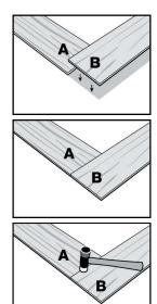
4. Position the long side of plank "B" over the short end of plank "A". Align the edge using the tongue of a spare plank. Tap the top of plank "B" using a soft-faced hammer to fully lock planks together. This step iscrucial for a good installation.
