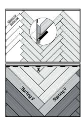
9. Measure, mark and cut planks that extend to the walls. Allow for 10mm spacers. A T-Bevel (angle finder) can be used to find the correct angle. Always measure twice before cutting. This is the last column of your installation, so all seams can be tapped to fully lock together at this time.
