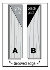
**3.** Separate "A" and "B" planks from the carton. If possible, install planks from 3 to 4 cartons at one time to ensure a mix of pattern and shade for best results. "A" planks have a pre-attached grey padding and "B" planks have a pre-attached black padding. Notice the groove edges are on the opposite long sides of the planks.
