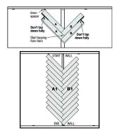
6. Continue to install column "A1" and "B1" as shown on the right. You should not tap down the last 51mm of the seam (in bold on the right). This space will be tapped and locked as the planks of the next column are added. Continue to ensure that your "starting V" is aligned properly (as described in Step 5) throughout the formation of column "A1" and "B1".
