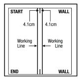
**2.** Measure 4.1cm from the left and right of the center mark. Snap chalk lines down the entire length of the room.
